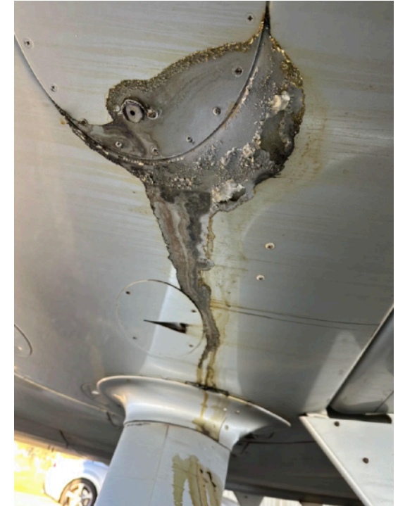
Paint damage on a Cirrus aircraft that started using G100UL.
