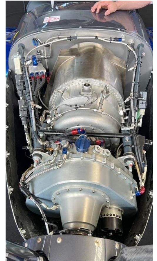
TurboTech has developed a highly efficient small gas turbine engine for use in Light Sport Aircraft.
